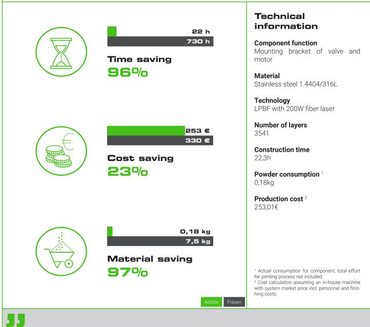
The component must withstand the engine torque and therefore have a high tensile strength. The material properties must ensure this.
