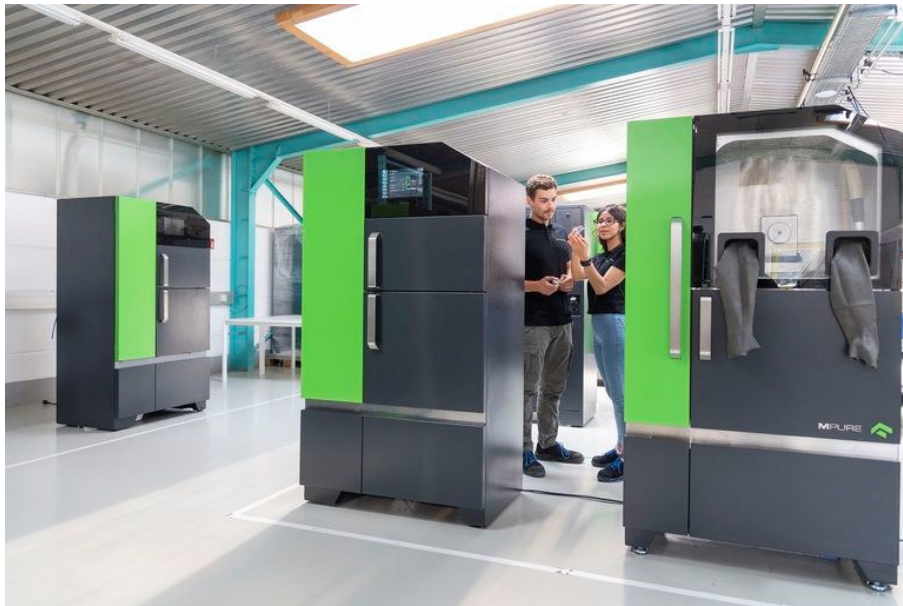
Photo 002: The Boldseries metal 3D printing solution consists of the MPRINT+ 3D printer, the MPURE unpacking station, which includes a sieving unit, and the MPREP data preparation software. Photo: One Click Metal GmbH
